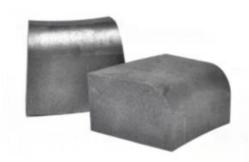
Graphite chill has a small proportion, about one-fifth of that of metal cold iron. Its fefractorinedd is as high as 2000 °C, high temperature resistance, not easy to oxidize, reusable and low cost. It is widely used in copper casting, cast steel and aluminum casting.
